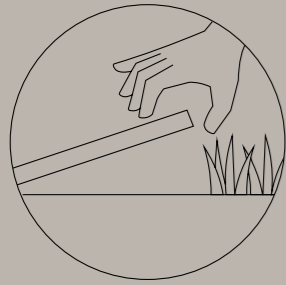
Posa su erba/ Dry laying on grass
